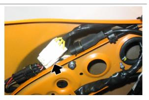
**2. Voltage regulator** - Remove the front central cover to reach it.
