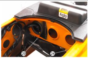
**25. Oil pressure sensor** - To access, remove the fan cover cap as described in the ENGINE chapter.
