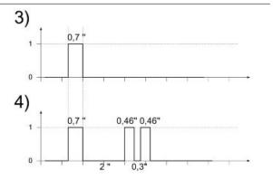
**5. Programmed control unit - fault detected**: a light code is displayed according to the fault detected, after which the LED remains on steadily. The engine cannot be started. The codes that can be transmitted are:
