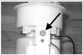
Remove the clip fixing the piping to the filter shown in the picture
