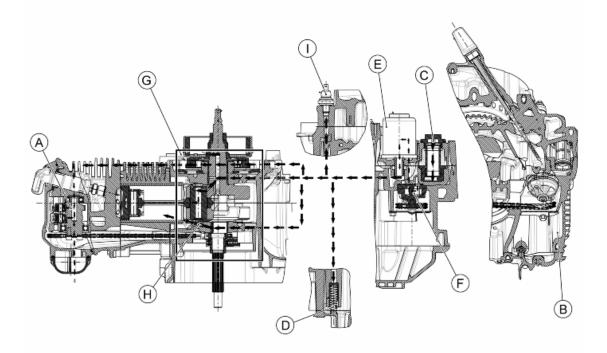
The lobe pump «F» sucks the oil from the sump, through the mesh pre-filter «C», it pushes it into the cartridge filter «E» where there is also a safety valve «D».
