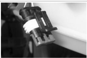
With the ignition switch at ON check there is battery voltage between the Orange-Blue and Black cables.
