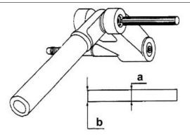
Use a suitable punch with the dimensions indicated on the figure; hit with a mallet until the wedging washer is crushed and then extract it with the help of a pointed end.
