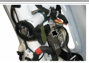
Remove the protective base from the connector.
