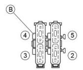
Check efficiency of the injection load relay, that can be reached by removing the central cover of the shield: check the resistance of the energising coil between pins 86 and 85: 40 to 80 Ohm Apply a voltage of 12V to pins 86 and 85; make sure that there is continuity between pins 30 and 87 of the relay.
