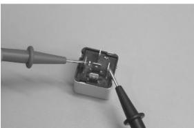
Check the presence of fixed voltage between the Red-White cable of the relay base and ground. Otherwise, check the continuity of the Red-White cable between the fuse-box (No. 6, 10 A) and the relay base.
