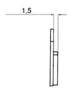
evenly. A 0.5 mm thickness difference in the residual friction material is permitted
