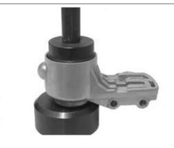
Assemble a new roller bearing on the shock absorber side and move it until it stops using the specific tool
