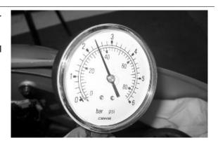
With the battery voltage > 12 V, check the pump flow rate by disconnecting from the injector the pipe equipped with the pressure gauge of the appropriate tool. Make a graded burette available with a flow rate of approximately 1 L. Rotate the pump using the active diagnosis of the palm top computer. Using a pair of long flat needle-nose pliers, choke the fuel pipe making the pressure stabilise at approx. 2.5 bar. Check that within 15 seconds the pump has a flow rate of approx. 110 cm<sup>3</sup>.
