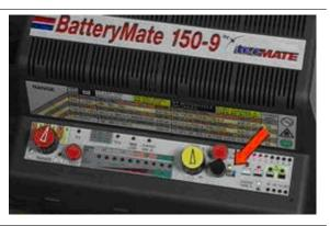
g - The activation cycle of the new battery lasts for30 minutes after the ignition of the recharge LED has taken place
