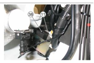
**29 - 24. Pump and fuel lever transmitter** - They are fitted on the tank, remove the fuel tank to reach them.
