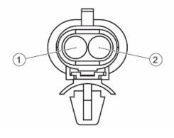
Short circuit to positive:excessive voltage at PIN 1 of the control unit connector.
