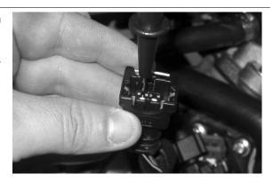
With injector disconnected and the injector load relay disconnected, check the continuity of the Black-Green cable between the injector connector and relay base.
