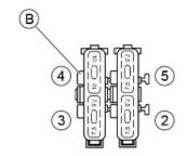
Check efficiency of the injection load relay, that can be reached by removing the central cover of the shield: check the resistance of the energising coil between pins 86 and 85: 40 to 80 Ohm Apply a voltage of 12V to pins 86 and 85; make sure that there is continuity between pins 30 and 87 of the relay.
