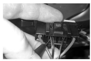
Switch to «ON» and check if there is voltage, with injector disconnected and control unit connected, between the Black-Green cable of the injector connector and the ground lead
