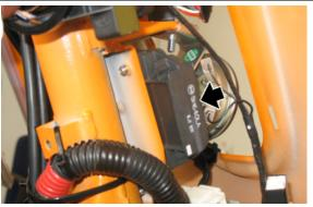
**3. Battery** - Lift the saddle and remove the cover to reach them.
