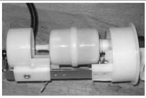
Remove the filter from the pump mounting
