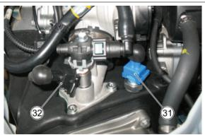
**33. H.V. coil** - Remove the helmet compartment and undo the two screws indicated to reach it.
